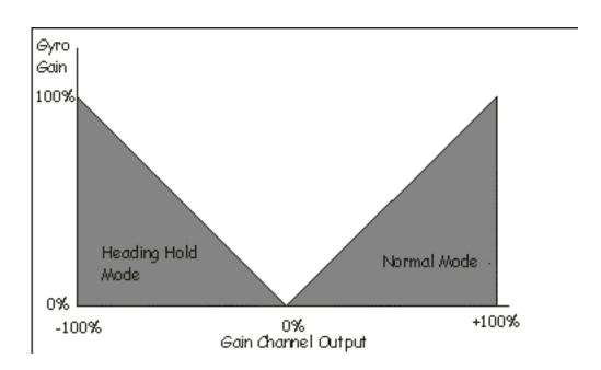
The next step is to trim the tail. This is done by switch the gyro between normal and heading hold and then watching the servo. Place the gyro in normal mode to center the tail servo. Now
